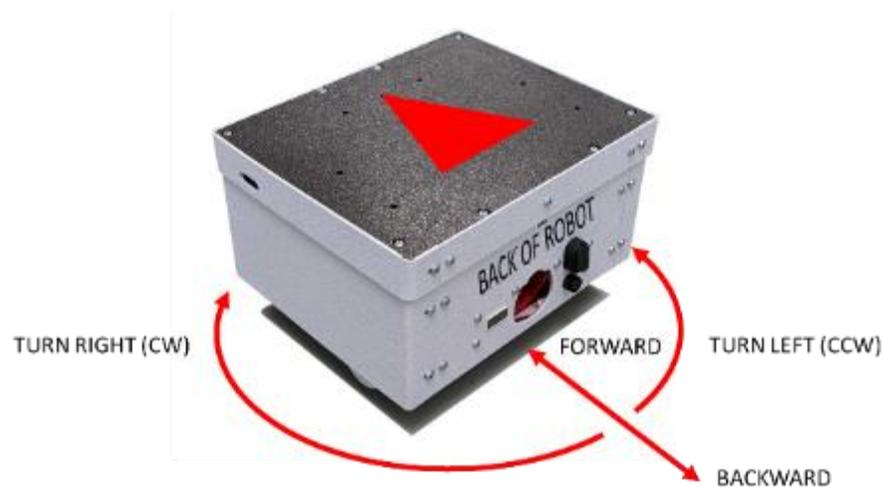
Driving the robot in **Joystick Mode** may require a little practice. The primary reason is that the forward/backward direction is defined relative to the robot, **not** the operator.
